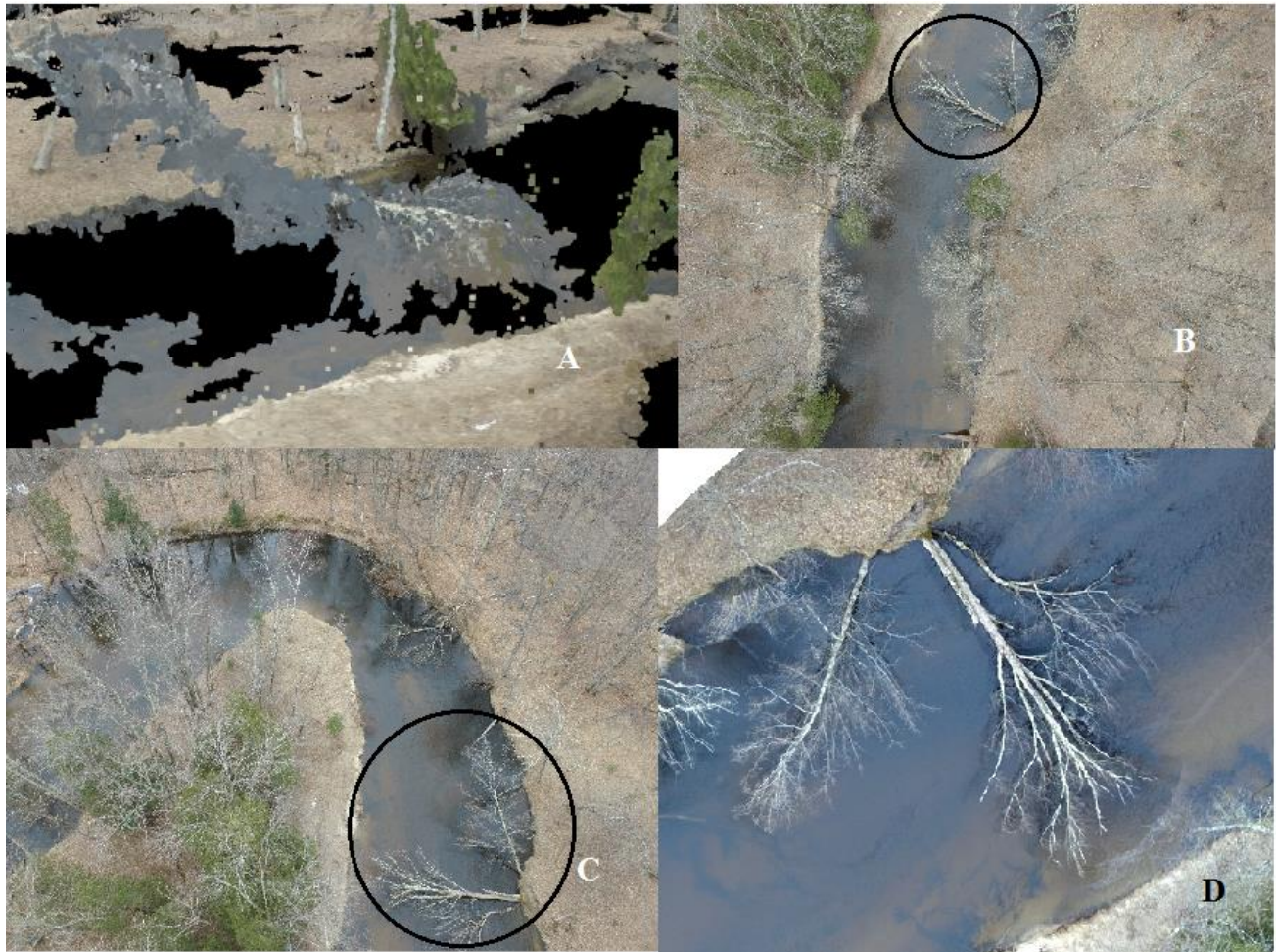
Figure 15: Examples of relief displacement. A) point cloud showing true verticality B) nadir image showing relief displacement C) oblique image showing true verticality D) orthomosaic showing relief displacement.
